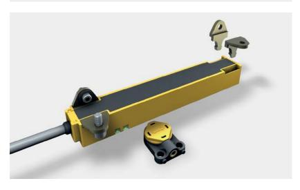
The compact Li-Q17L as well as the Li-QR14 series are built in a highly tight plastic housing, made for many aggressive ambient conditions. They are available in lengths of 50 mm to 300 mm (Li-Q17L series) resp. 25 mm (Li-QR14 series). Angled and straight mounting elements guarantee highest flexibility for mounting. The positioning element is moreover rotatable and can be oriented parallelly or crosswise to the sensor.
